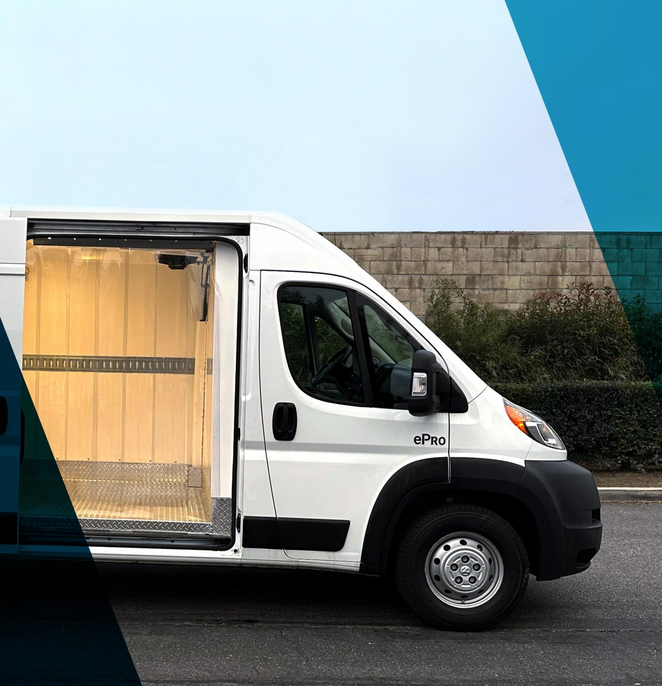
The ePro Cooler is an electric reefer van with 150 miles of range featuring an integrated refrigeration system powered by the EV battery. The 120-hour, no-idle runtime keeps up to 3,000 lbs of cargo as cool as 32°F with automatic defrost and open-door shut off to save energy. A 30 minute recharge puts long routes in reach, while networked controls help the ePro work for your fleet.
